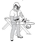
4 Never use the chain saw above shoulder height and avoid cutting with the tip of the bar. Never use the chain saw one-handed!
